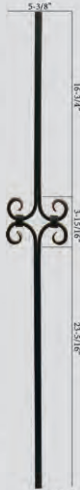
HF 16.8.8 Ends : 5/8" Sq. Height: 44" Wt. 3 lbs. TUBULAR
