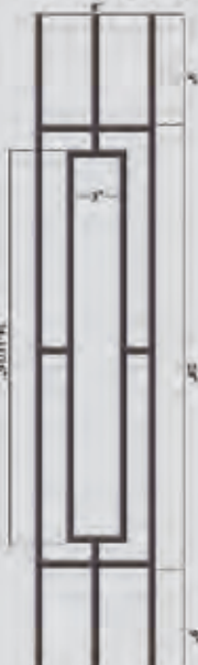
HF 9.4.11 Ends: 1/2" Sq. Height: 46" Wt. 4.5 lbs. TUBULAR (Rake)
