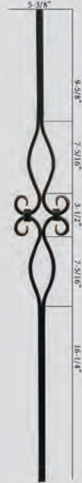
HF 16.8.9 Ends : 5/8" Sq. Height: 44" Wt. 4 lbs. TUBULAR
